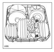
The rows of prongs on the lower basket can be easily lowered to allow you to load pots, pans and bowls.
